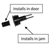
14. Swing Door Interlock Kit – For Doors Leading Into the Lift Area Electrical Interlock kits retrofit into most single-swing doors, and include a locking mechanism and a status switch. The switch senses if a door is left open and, if so, prevents the lift from operating. The lock automatically engages whenever the lift is in motion to prevent a closed door from being opened.
