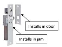
15. Overhead door interlock kit – For Doors Leading Into the Lift Area Electrical Interlock kits retrofit into most overhead doors, and include a locking mechanism and a status switch. The switch senses if a door is left open and, if so, prevents the lift from operating. The lock automatically engages whenever the lift is in motion to prevent a closed door from being opened.
